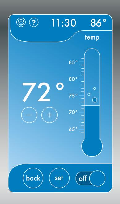
To change the temperature you would be able to slide your finger along the thermostat or use the plus and minus buttons.
